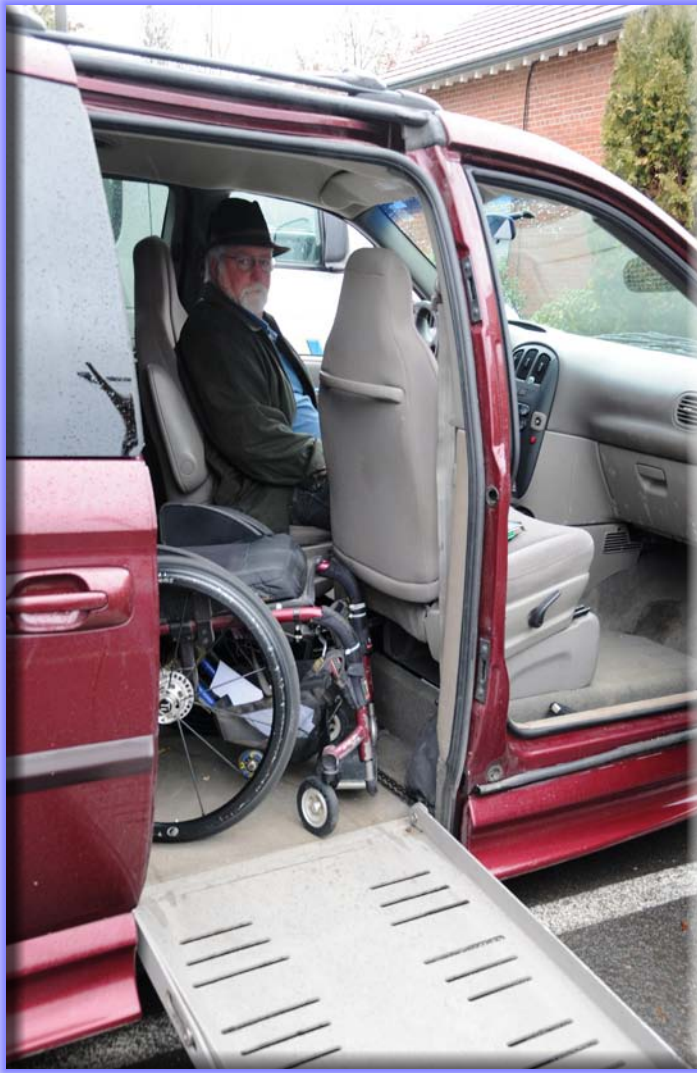
Pictured: Michael Gardner shows off his Van's super technology by pushing a button that lowers the right side of the vehicle. He then flips a switch and the door opens and the ramp drops down. Mike swivels the driver's seat around to maneuver himself into the waiting wheel chair, and traverses the ramp. Once he is out of the vehicle, he pushes another button adjacent to the van door and the ramp flips up and the door closes. Amazing!
