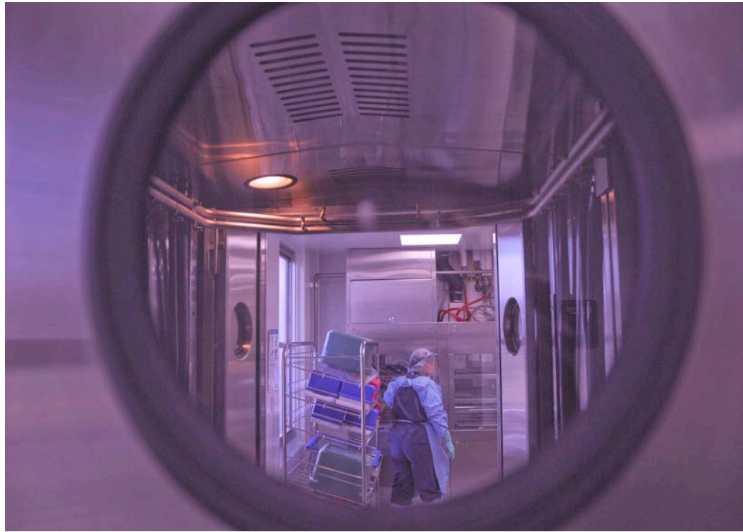
The SPS Cart Washer is a state-of-the-art piece of equipment with doors on both sides. Roll in the cart from one side, sterilize, and remove cleaned scopes etc, from the other. Pictured: Lynne White through the Cart Washer door.
