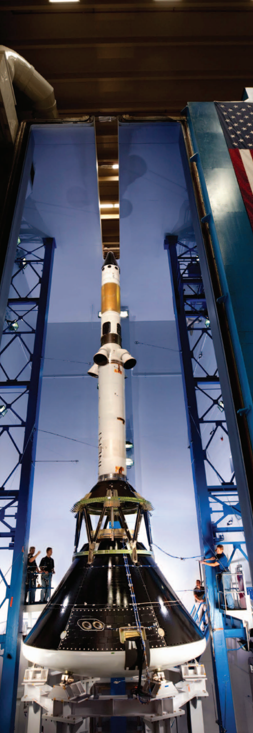
Technicians position microphones around the Orion Multi-Purpose Crew Vehicle and the Launch Abort System in preparation for a second round of acoustic-chamber testing. (Lockheed Martin)
