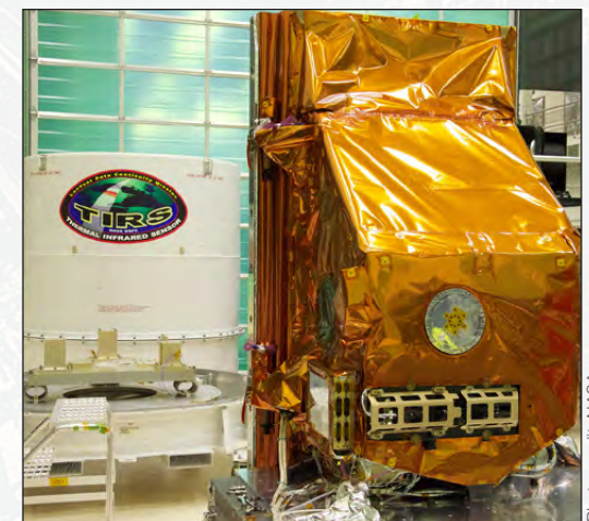
The TIRS instrument, built in-house at NASA's Goddard Space Flight Center, uses a new technology that is sensitive to two thermal infrared wavelength bands—an advancement over the single thermal band data collected by previous Landsat satellites.
