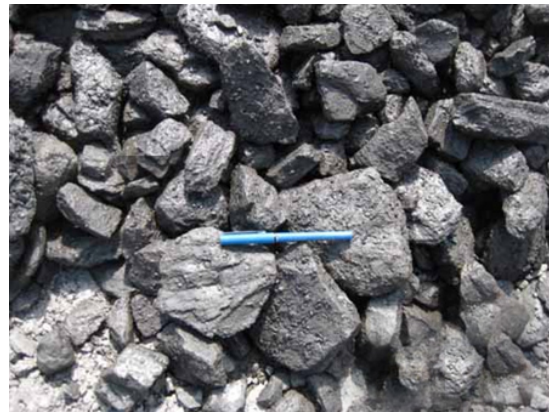
Example 2: Shows how using an ink pen approximately 5 inches long clearly shows that the coarse refuse exceeds the two-inch size limit.
