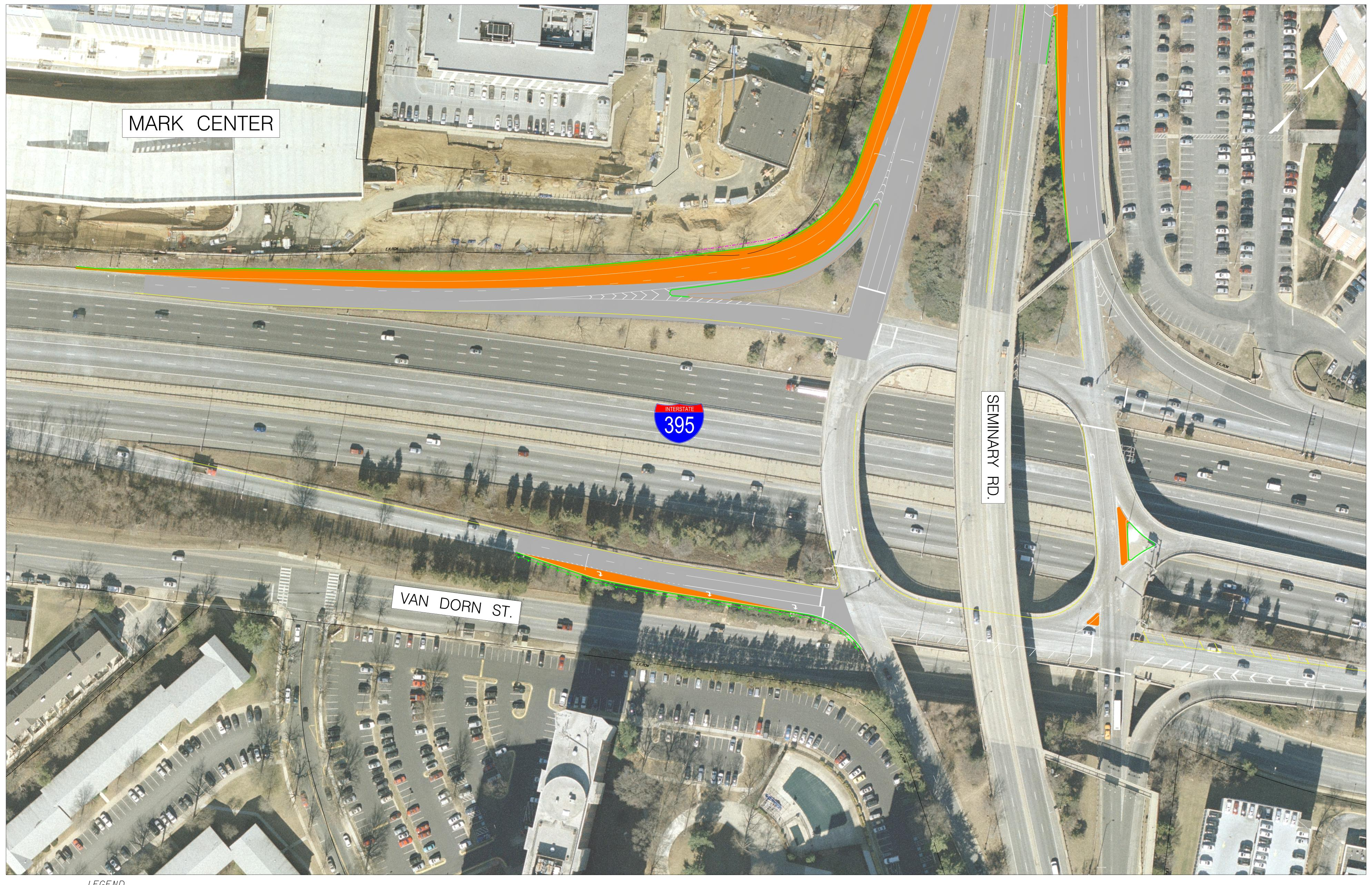
LEGEND ASPHALT PAVEMENT WIDENING ASPHALT PAVEMENT OVERLAY \_\_\_\_\_ EXIST. R/W CONCRETE SIDEWALK PROPOSED PEDESTRIAN BRIDGE
