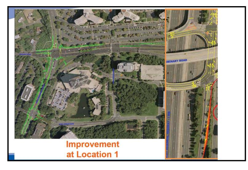
**Location 1** Widen northbound I-395 off ramp from 2 to 3 lanes and provide two through lanes and one right turn lane. Restripe the rotary to provide dual lefts for the northbound to westbound movements and eastbound to northbound movements. Restripe the westbound movement to provide two through lanes and one southbound left turn lane.
