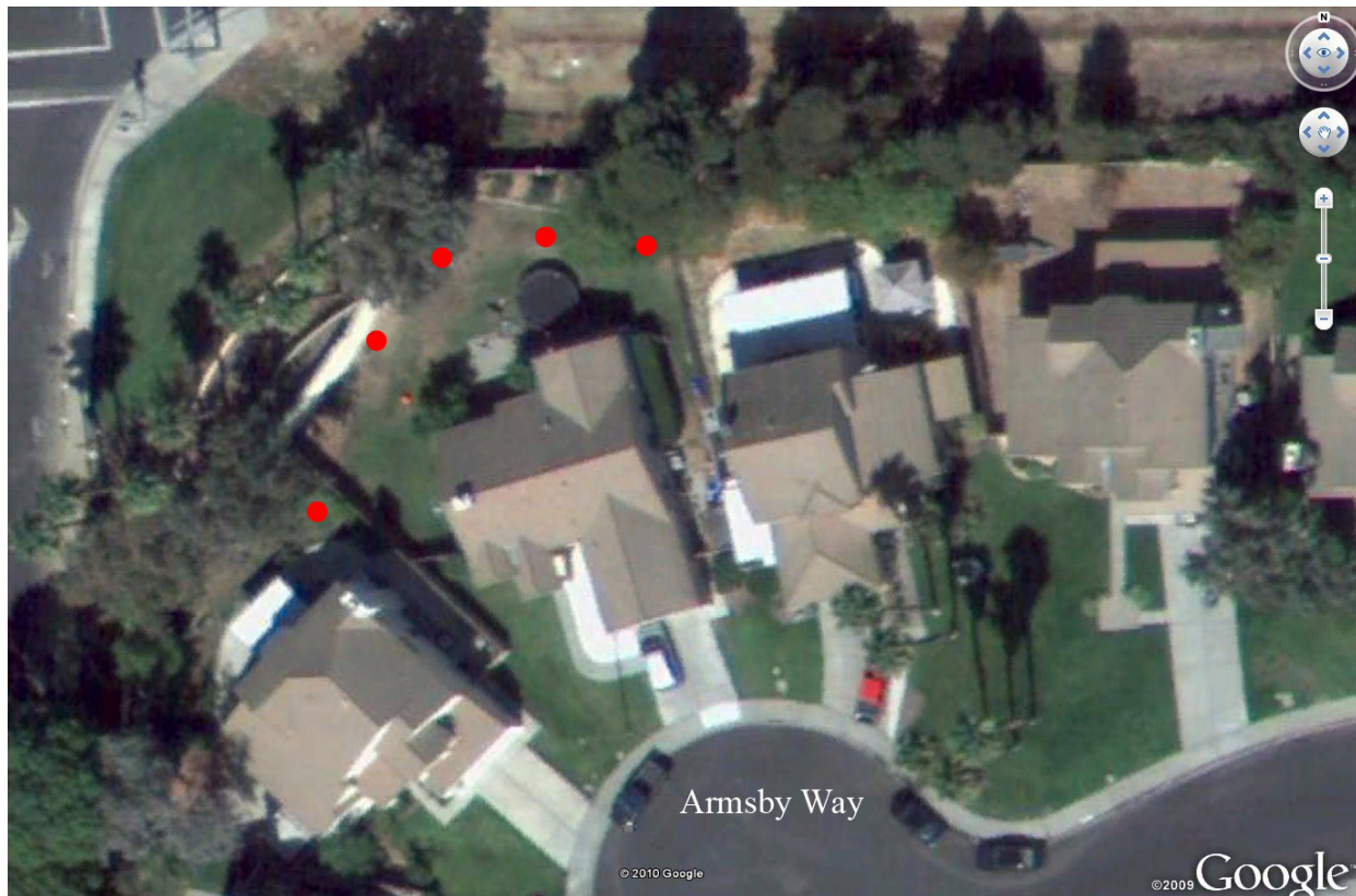
Overhead view of the southern part of the Jet Fuel Leak Area. The red dots represent the highest fuel concentrations found in subsurface soil samples.
