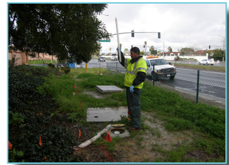
A field technician inspects a groundwater sample in a bailer. Visual inspections of water samples from monitoring wells identified the presence of fuel on the water table.
