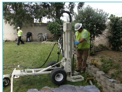
A drilling specialist uses a mobile Geoprobe drill rig to collect soil samples. This type of sampling equipment works well in confined spaces and areas with limited access.
