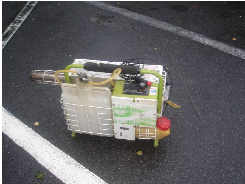
Photo 7: Odour treatment can be carried out using a so-called fogger. The machine is a kind of petrol-driven jet engine, where the scent is added under pressure to the engine's exhaust pipe, generating a fog of small particles in the air.
