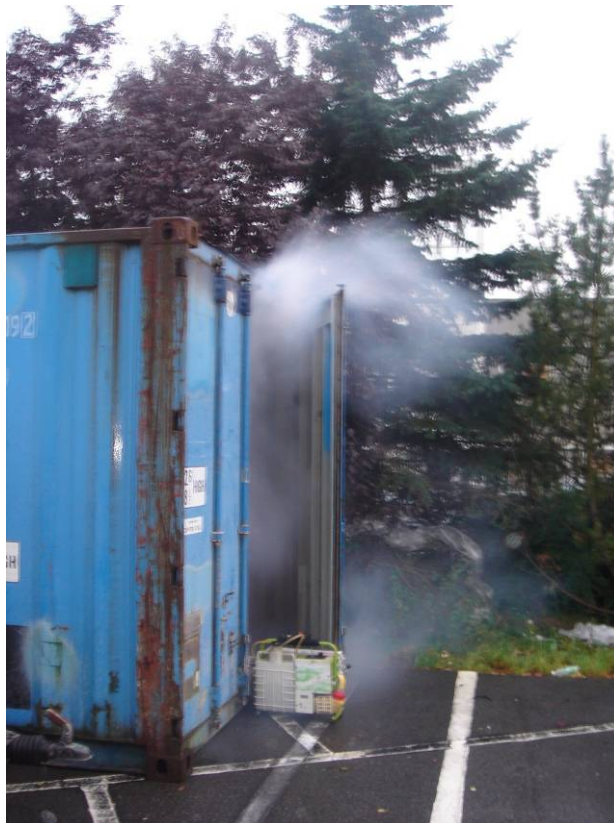
Photo 8: Movables with a smell of smoke is being treated in this container. Note the strong development of smoke from the fogger.
