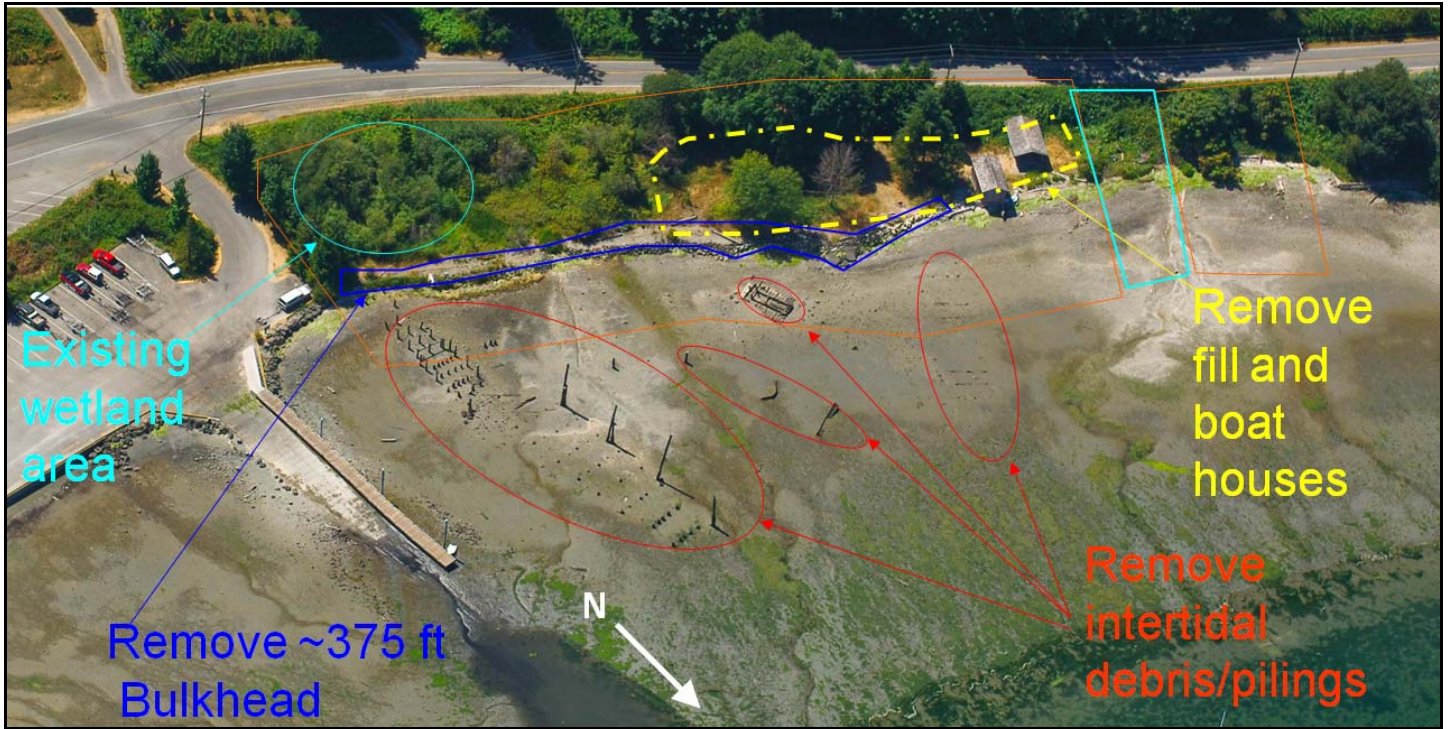
Figure 8 Dockton Major Restoration Components
