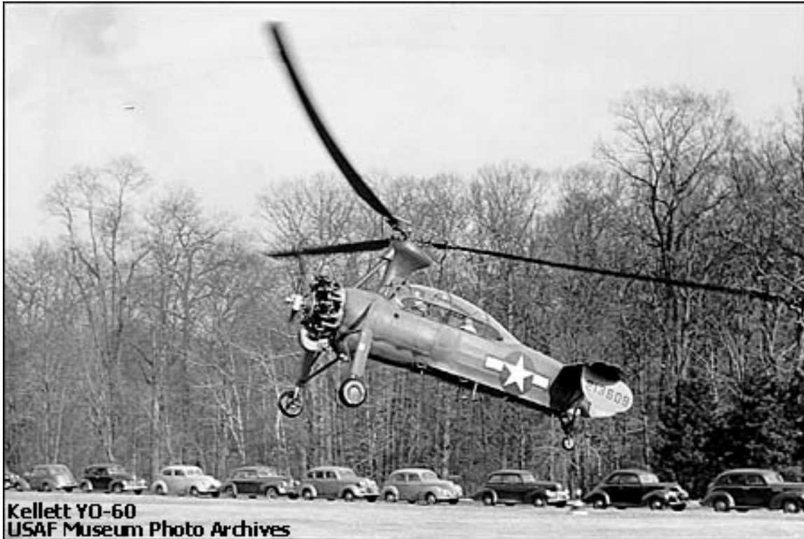
Kellett YO-60 USAF Museum Photo Archives US Army Air Corps Kellett YO-60 Autogiro with Plexiglas canopy for observation trials, 1942-43.
