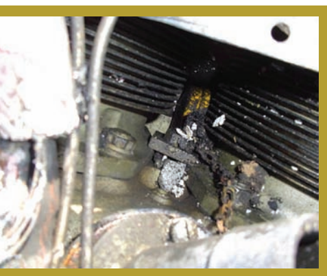
The Cessna 210’s oil filler cap was found unsecured between cylinders 4 and 6.
