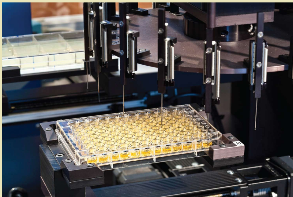
Automated Microbial Colony Picker at GLBRC. GLBRC screening efforts begin with the automated selection of microbial colonies in multiwell plates—selecting up to 7,000 colonies per hour. The robot then dispenses growth medium into the destination plates and seals the plates for analysis. [Photo by Wolfgang Hoffmann, University of Wisconsin–Madison]
