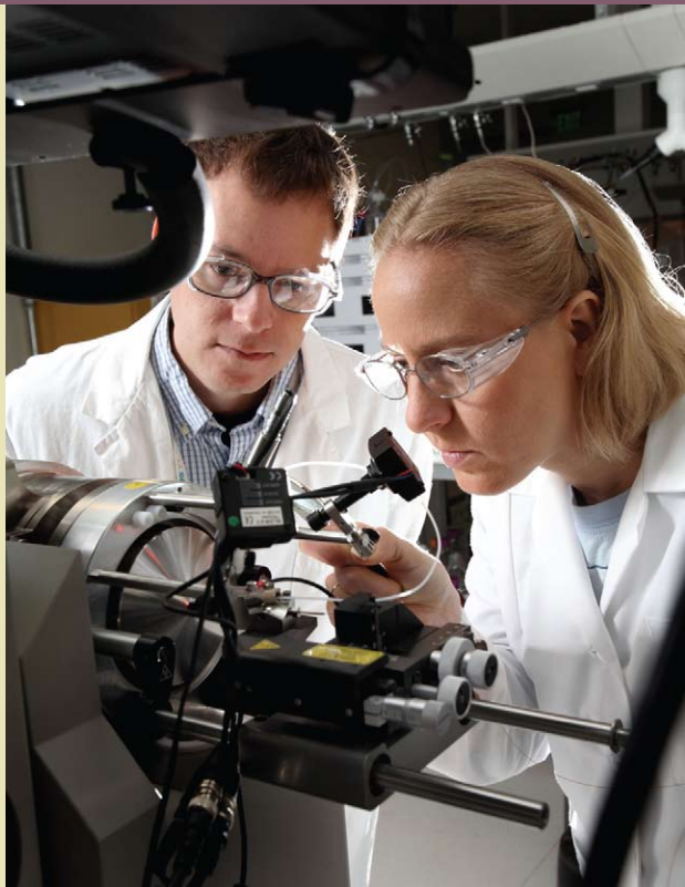
JBEI Technology Development to Advance Biofuel Research. JBEI's Chris Petzold and Alyssa Redding develop and apply mass spectrometry approaches to sort through the complex protein mixtures in biological cells and detect multiple target proteins in the same sample. [Photo by Dino Vournas, Sandia National Laboratories]
