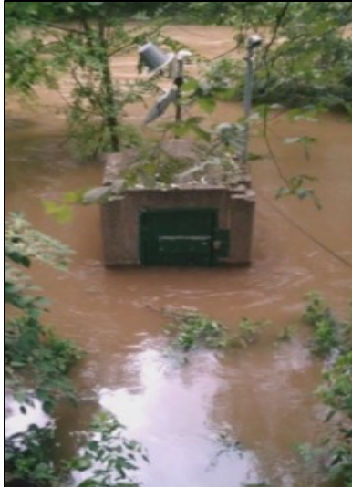
Figure 15: Flooding at the USGS gage on the Saddle River at Lodi, NJ, after the peak measurement on August 28, 2011. (Source: John Trainor, USGS)
