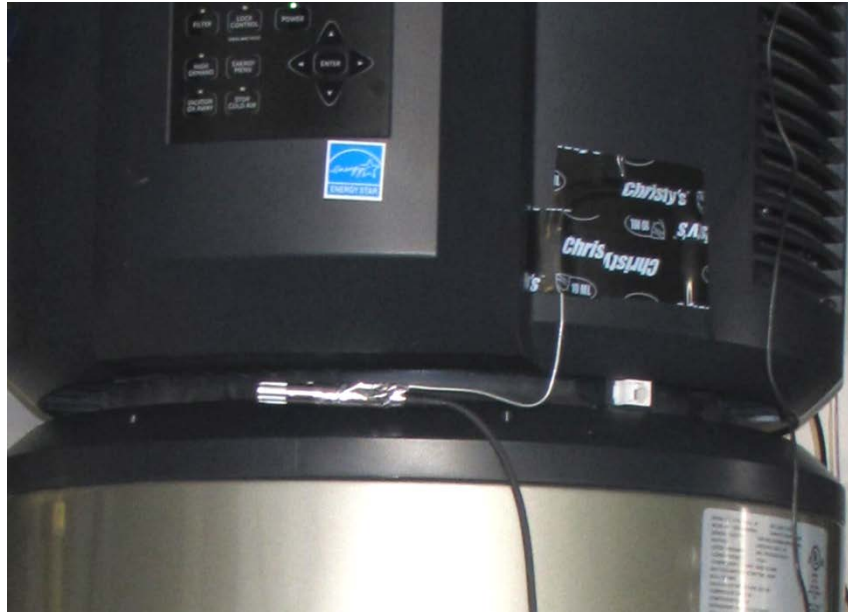
Figure 23. T&RH sensor is mounted on the front of the HPWH to measure inlet air conditions.
