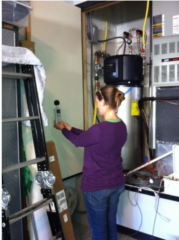
Figure 27. Performing a sound test for the HPWH
