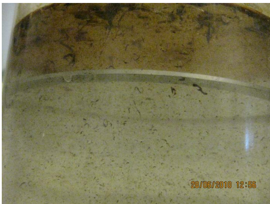
Figure 4.7 Droplet formation in the IFP test with the emulsion from position 3. The test is performed with Corexit 9500 and DER=1:25.
