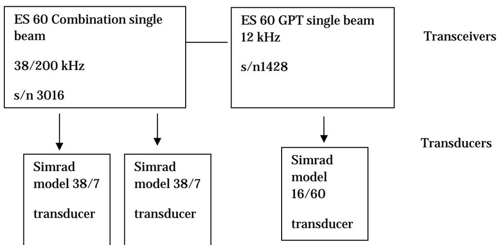
**Figure 1: Block diagram of Simrad ES60 installation. Serial numbers for the transducers were not available.**
