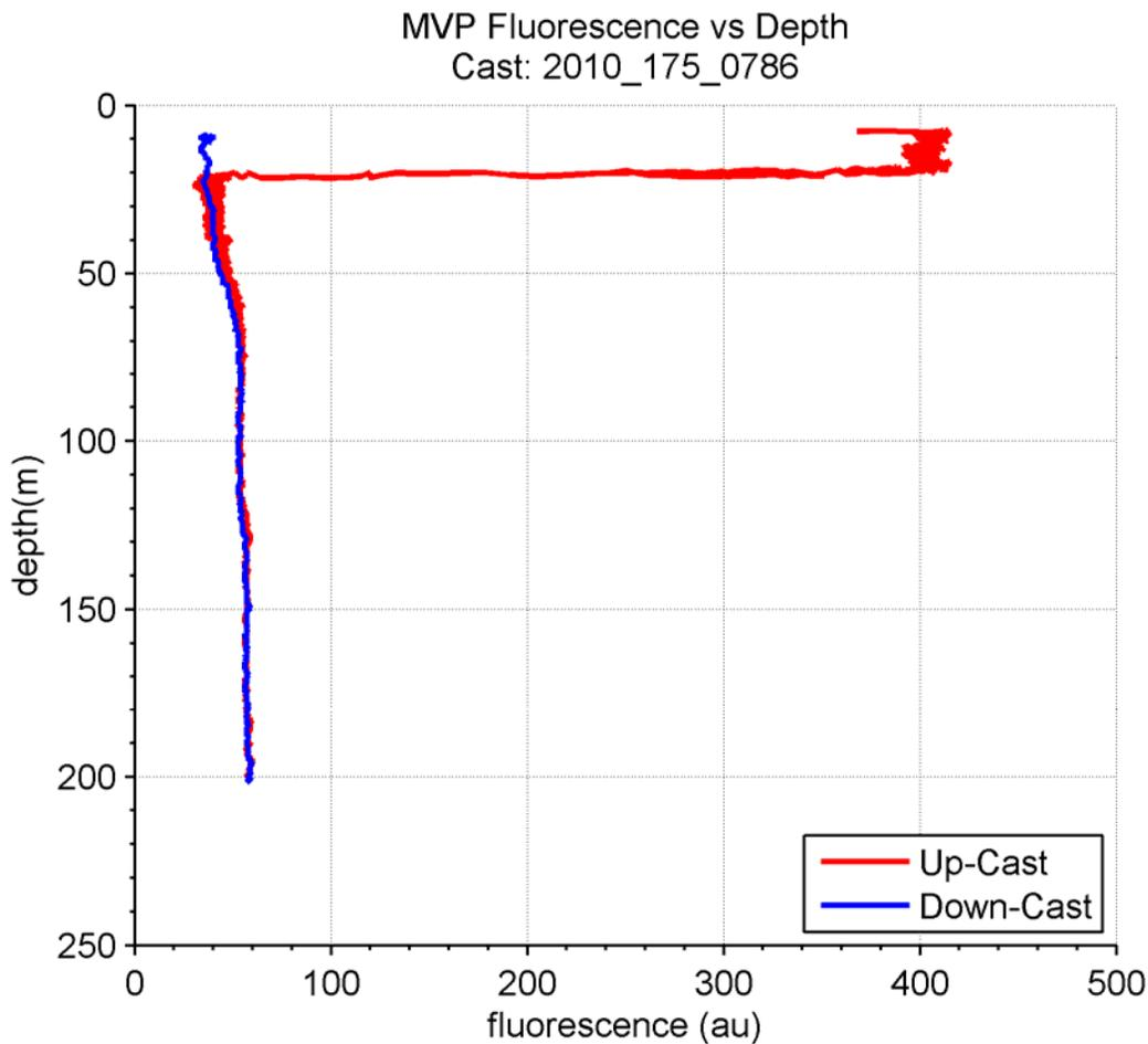
**Figure 7: Anomalous reading on up-cast of MVP mounted fluorometer not present in down-cast.**
