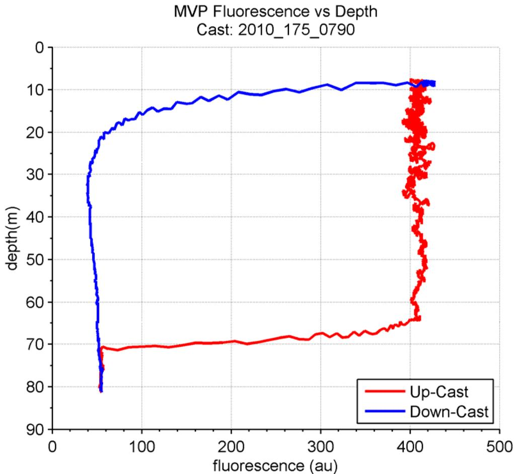
**Figure 9: Near surface fluorescence anomalies in both up-cast and down-cast data. Up-cast anomaly is suspected to be due to sunlight. Down-cast anomaly may be due to system latency.**
