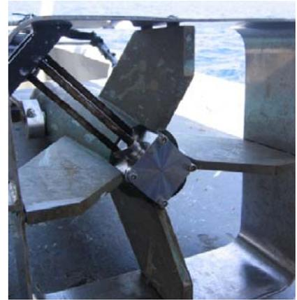
**Figure 3: AML SV&P sensor (on single sensor fish)**
