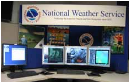
AWIPS Linux workstation consisting of single-screen text workstation and a triple-screen graphical workstation
