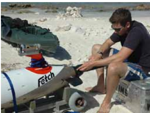
Daniel Jones preparing to launch the Fetch autonomous underwater vehicle (AUV). He is attaching Fetch's "nose," which contains the side scan sonar, some of the water quality sensors, and the color video camera. Image courtesy of Bonaire 2008: Exploring Coral Reef Sustainability with New Technologies.
