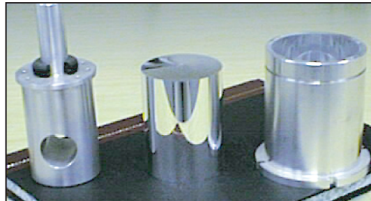
Simultaneous small-angle neutron scattering and rheology for bulk shear effects.
