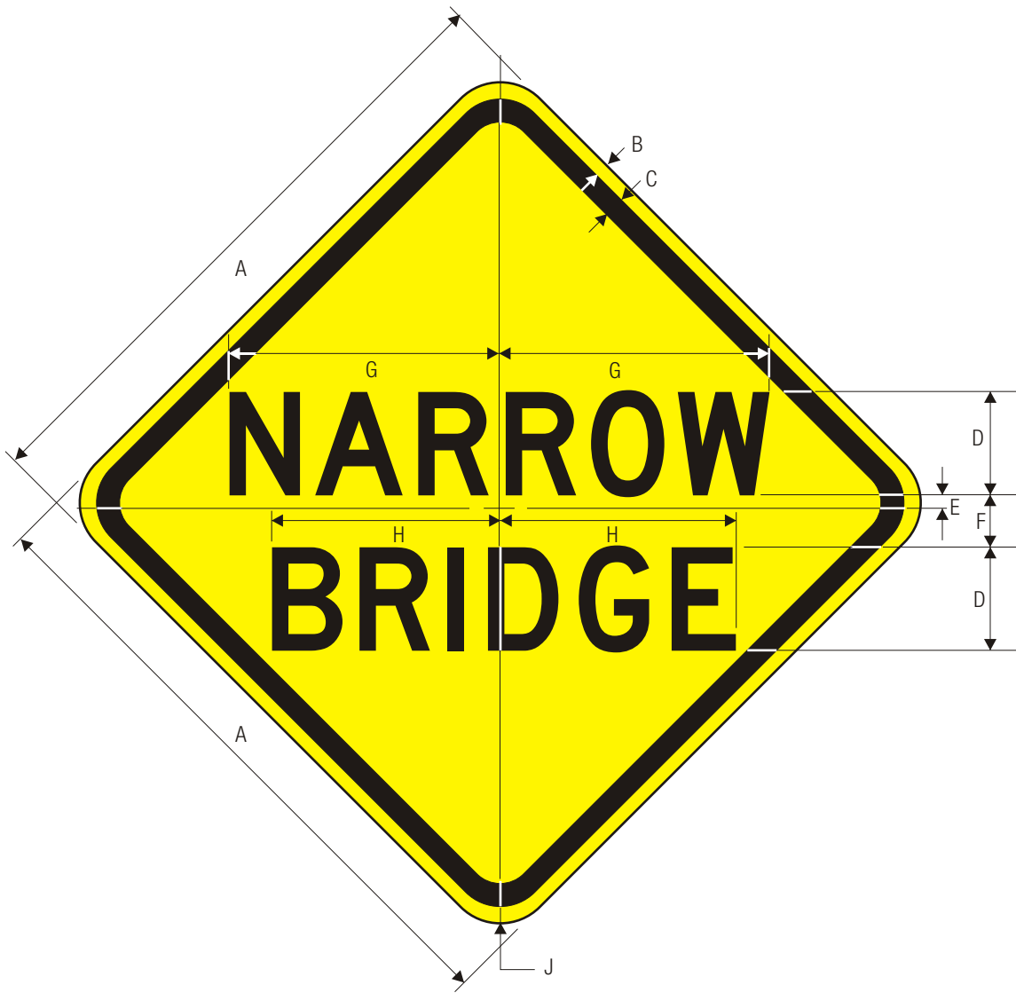
W5-2 NARROW BRIDGE
