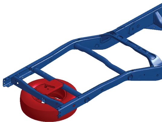
Figure 7.21. Spare tire and its carrier (denoted by the red color).
