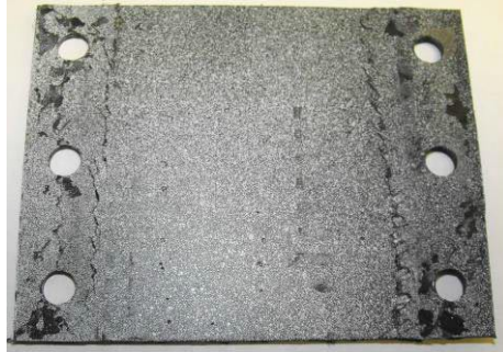
Figure 56. Typical Failure Location for Transverse Compressive Specimens
