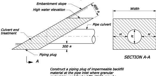
material is used for backfill. Width may be adjusted to tie into impervious material.
