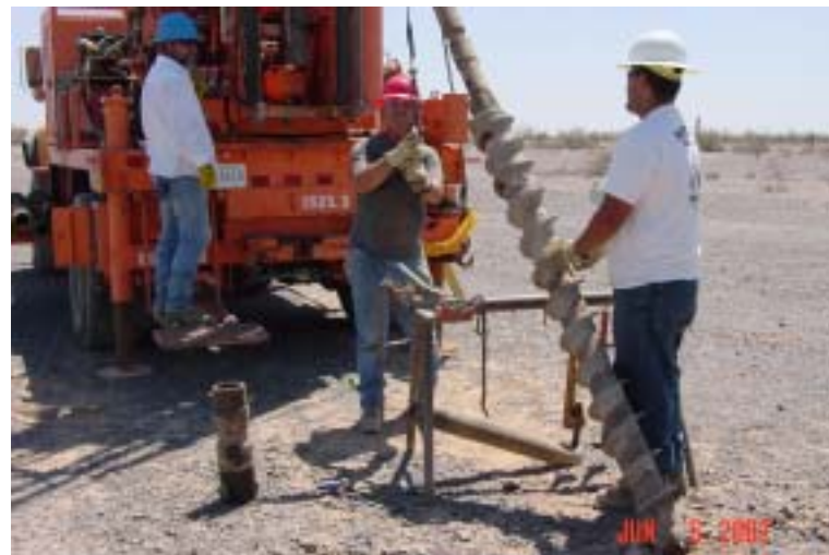
Figure 3. Pictures of drill rig and hollow stem auger used to retrieve soil cores
