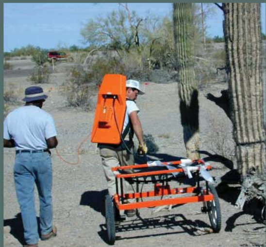
A team tests a prospective UXO detecting system on the Standardized UXO Technology Demonstration Site at Yuma Proving Ground, Arizona.
