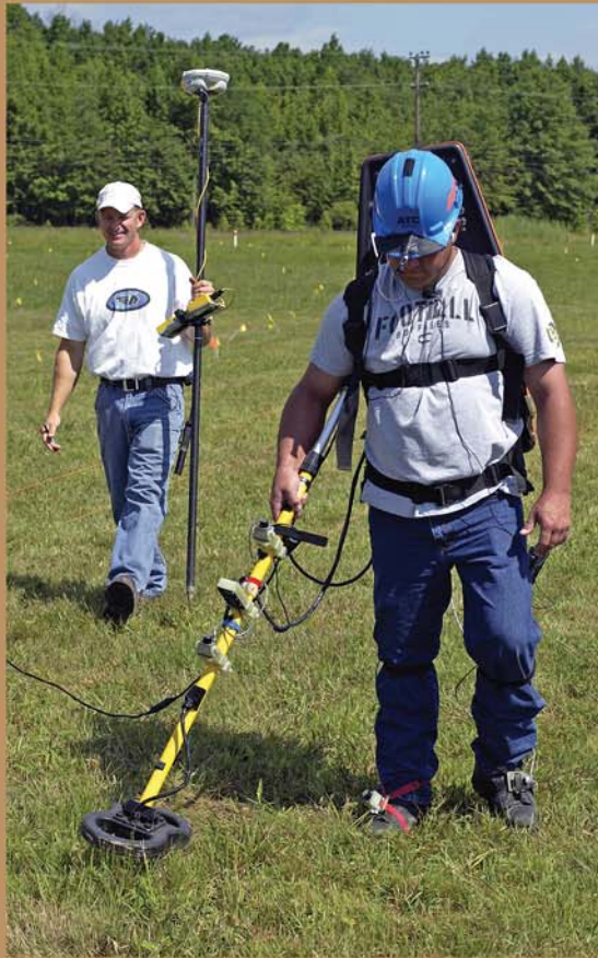
Team evaluates a UXO technician at the Aberdeen Test Center to determine degree of operator influence.
