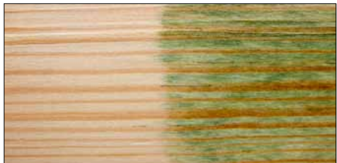
Figure 31. A water-based copper naphthenate solution (1% copper) was applied to the right side of this specimen and allowed to dry before this photograph was taken.
