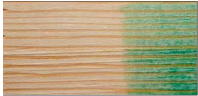
Figure 29. A solvent-based copper naphthenate solution (1% copper) was applied to the right side of this specimen and allowed to dry before this photograph was taken.
