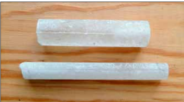
Figure 28. Borate rods are available in a range of sizes including the 19-mm (0.75-in.) and 13-mm (0.5-in.) diameters shown here.
