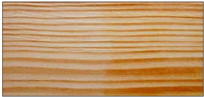
Figure 25. A 22% DOT glycol–borate solution was applied to the right side of this specimen and then allowed to dry before this picture was taken.
