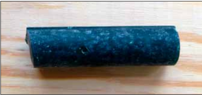
Figure 27. Example of 19-mm- (0.75-in.-) diameter rod that contains both copper and boron.
