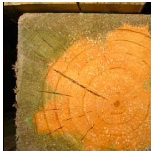
Figure 7. During pressure treatment, preservative typically penetrates only the sapwood. Round members have a uniform treated sapwood shell (upper photograph), but sawn members may have less penetration on one or more faces (lower photograph).
