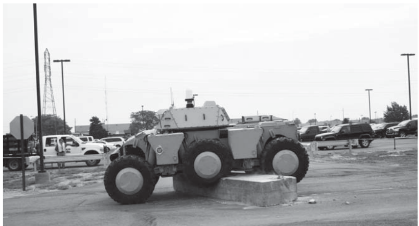
An APD maneuvers over concrete blocks outside of a TARDEC building at the Detroit Arsenal. The APD is helping TARDEC engineers develop, integrate and test next-generation UGV mobility technologies. (U.S. Army TARDEC photo by Carolyn Baum.)
