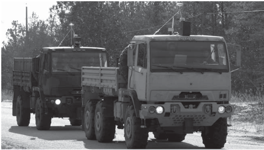
The ANS is an onboard, integrated suite of sensors and technology that enable autonomous navigation, perception, path-planning and vehicle-following capabilities for UGVs, allowing them to move on the battlefield with minimal human oversight. (Photo courtesy of PEO I.)
