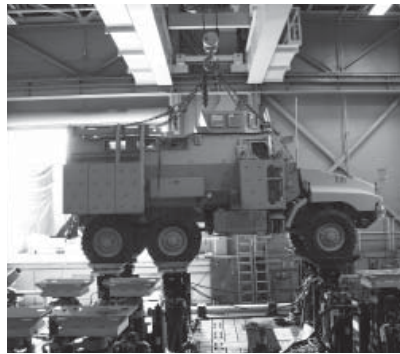
Vehicle testing is a key component service that TARDEC provides to the TACOM LCMC and its respective PEOs and PMs. Testing results provide crucial information necessary for decision makers to make informed engineering and integration decisions. Here, an MRAP vehicle is tested on TARDEC's Reconfigurable N-Post Simulator. (U.S. Army photo by Carolyn Baum.)
