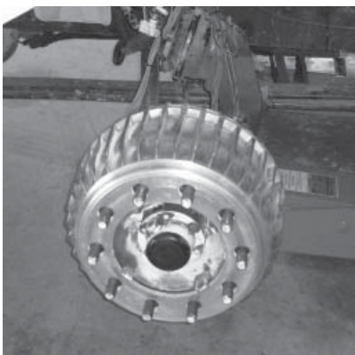
This new lightweight brake drum manufactured by Century, Inc. is one of many items being considered for vehicle weight reduction. (Photo courtesy of Century, Inc.)
