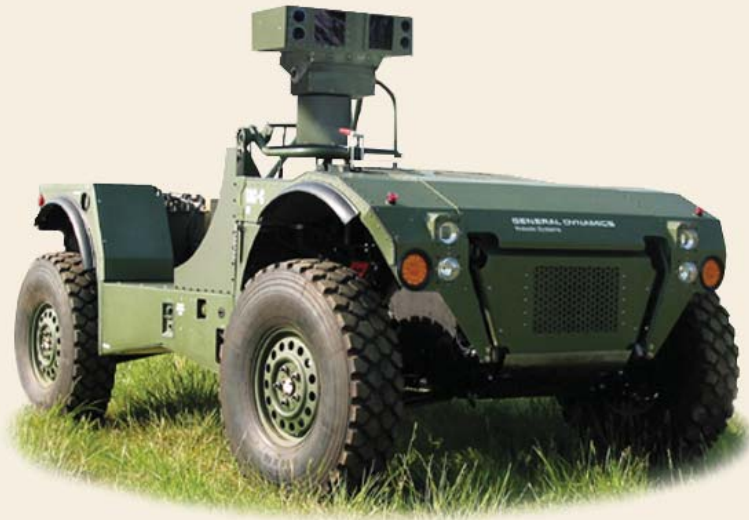
General Dynamics Robotic Systems' (GDRS) Tactical Autonomous Combat – Chassis vehicle, part of the ANS system. GDRS is responsible for the design, development, manufacture, integration and testing of the ANS for the Army's BCT Modernization Plan. The ANS system is capable of autonomously controlling any of several vehicles designated by the Army, including the Multi-functional Utility Logistics Equipment platform, the Armed Reconnaissance Vehicle and manned ground vehicles. (Photo courtesy of GDRS.)
