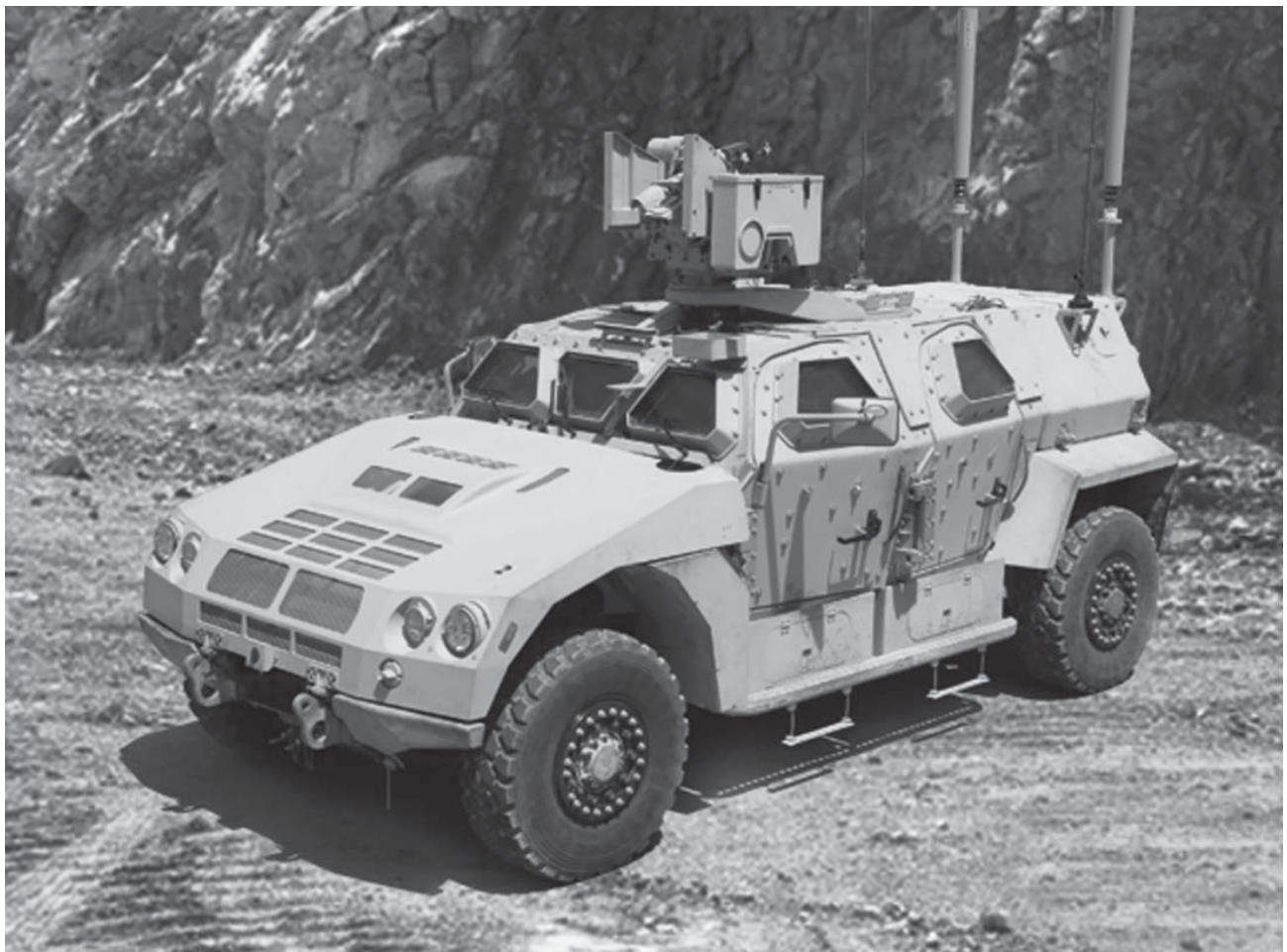
BAE Systems’ JLTV design incorporates lessons learned from DOD’s Mine Resistant Ambush Protected vehicle program and features the latest in lightweight, advanced armor and a V-shaped hull design to provide maximum crew protection against mines and IEDs. (Photo courtesy of BAE Systems.)
