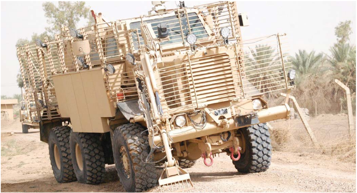
Soldiers use a Buffalo MRAP vehicle to clear a lane during route clearing training at Victory Base Complex, Iraq. The Soldiers learn to operate the Buffalo's mechanical arm and other specialized equipment during the training in preparation for real-world route clearance and convoy operations. The LCMC has recently placed an emphasis on route-clearance systems as a direct response to threats Soldiers face every day in the field. (U.S. Army Multi-National Division Baghdad photo by SGT Tracy Knowles.)
