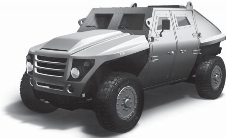
This concept drawing of the Ricardo-designed FED offers a designer's rendering of how the vehicle may look upon completion. After thousands of models and countless hours of analysis, the program is proceeding to design and build a vehicle capable of dramatically improving fuel economy in the field. (Image courtesy of Ricardo plc.)
