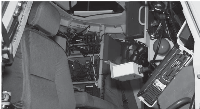
The ISD cockpit is crammed with technology. Each piece of equipment was carefully positioned after a detailed human factors analysis. The ISD crew compartment will continue to be modified with future Soldier-in-the-loop training to make the system as user-friendly as possible. (U.S. Army TARDEC photo.)
