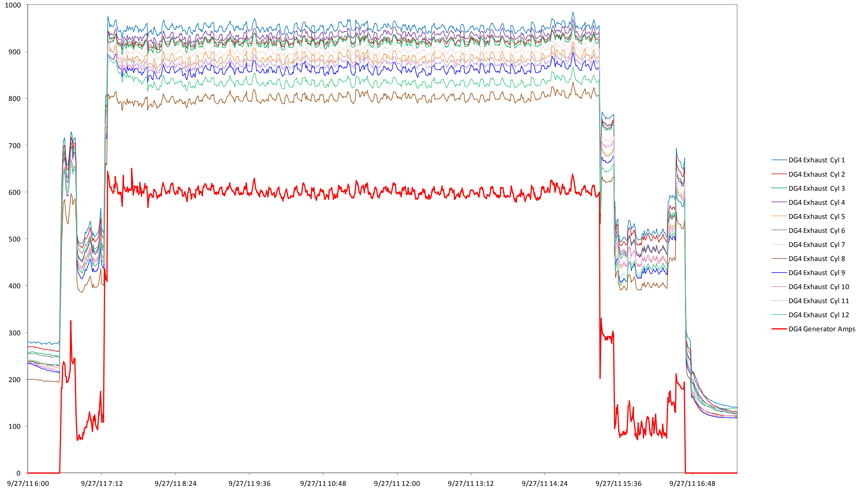
Diesel Generator #4 Exhaust Cylinder Temperatures and Generator Amps – September 27, 2011 Test Data Close-Up
