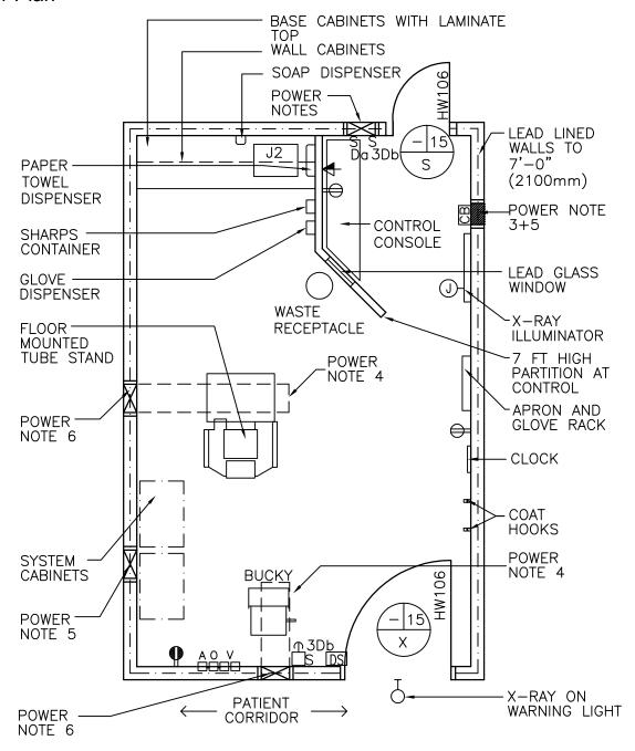
NOTE: RADIOLOGY EQUIPMENT LAYOUT SHOWN IS TYPICAL, EXACT EQUIPMENT LAYOUT SHALL BE COORDINATED WITH RADIOLOGY EQUIPMENT MANUFACTURER/PROVIDER.
