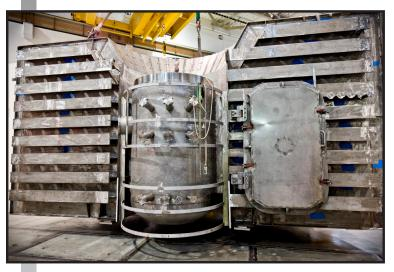
instrument combines the high efficiency of whitebeam Laue diffraction with energy discrimination by modulating the beam with a statistical chopper. A cross-correlation method is used to reconstruct the elastic signal from the modulated data. Accurate modeling of the shortrange order associated with the diffuse scattering requires measurements over large volumes of threedimensional reciprocal
