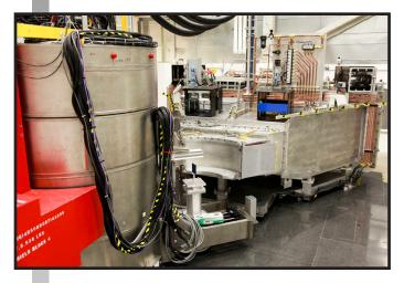
optics, plus a position-sensitive detector bank, leads to a highly flexible instrument in which the energy and wave vector resolution can be independently varied by nearly an order of magnitude. Either full or partial neutron polarization analysis can be deployed on HYSPEC. This is accomplished by using a Heusler crystal array to polarize the incident beam and either a <sup>3</sup>He spin filter or supermirror wideangle polarization analyzers for the scattered beam.
