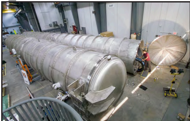
Detector tanks for the SANS instruments at HFIR. The Bio-SANS detector is on the left.
