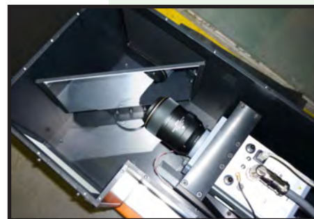
Detector housing for the CCD camera lens, mirror, and scintillator.
