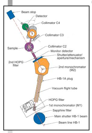
neutrons:  $I_{\chi 2} \approx 10^4 \times I_{\lambda}$ . This spectometer also has one of the most intense beams at this energy at HFIR, as well as a very low  $\gamma$  and fast neutron background. Typical energy resolution is  $\sim 1$  meV, but, using the beryllium analyzer, the energy resolution width can be reduced to  $\sim 0.5$  meV.
