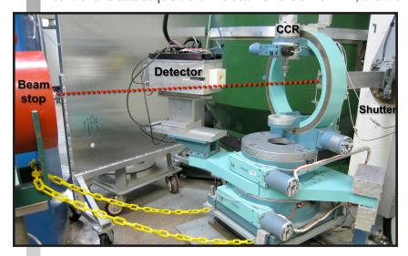
size is 1 mm<sup>3</sup>. The maximum crystal dimension is about 4 mm. The flux on the sample is up to  $2.2 \times 10^7 \,\text{n/cm}^2/\text{s}$ . Both high-resolution or high-intensity modes are possible by tuning the horizontal bending of the monochromator.
