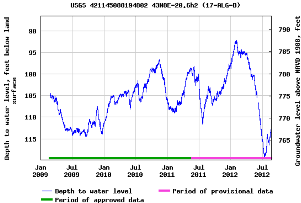
Figure 6. Graph showing a large decline for most of 2012 in groundwater level for a well near Lake in the Hills, McHenry County.
