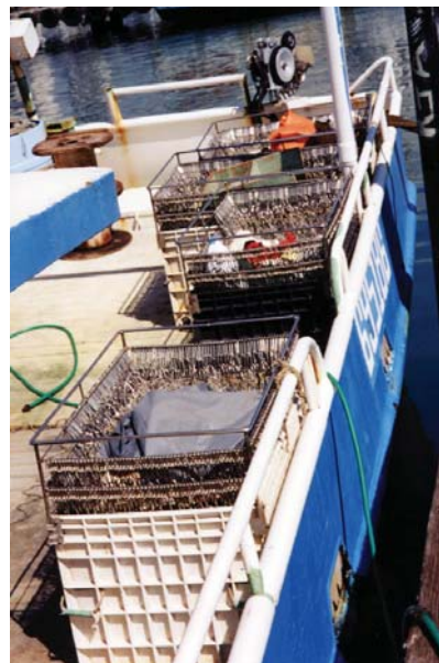
Hook storage bins and line shooter on stern of longline boat
