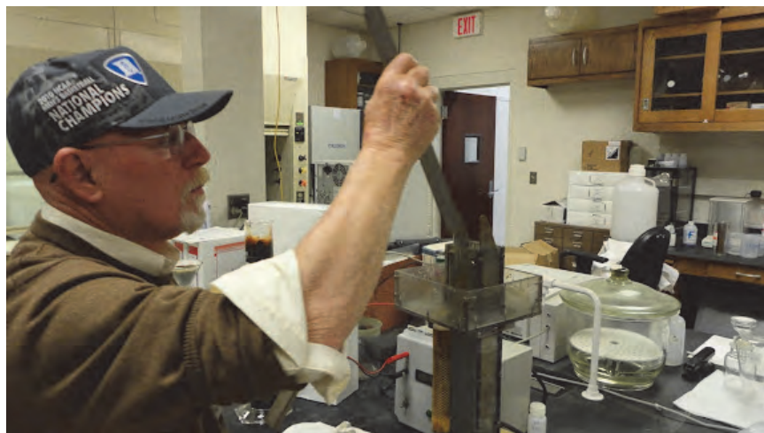
Figure 4. Setup of bench-top electrocoagulation unit.
