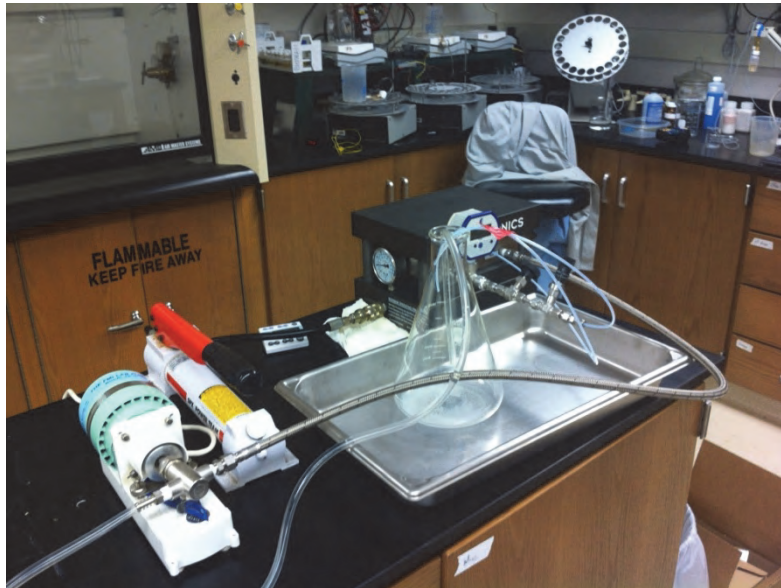
Figure 6. The experimental reverse osmosis reactor setup.
