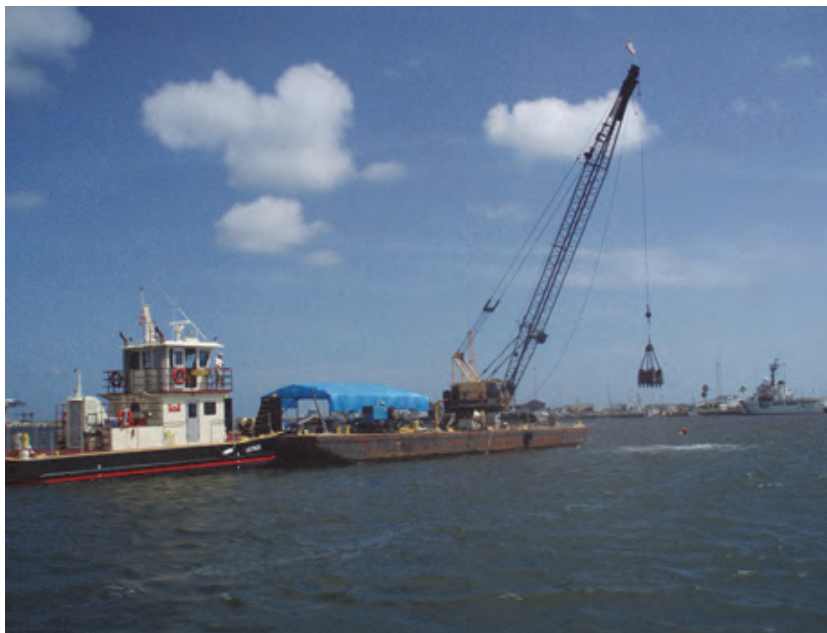
Figure 5. Bucket dredge equipment used in simulated operation.
