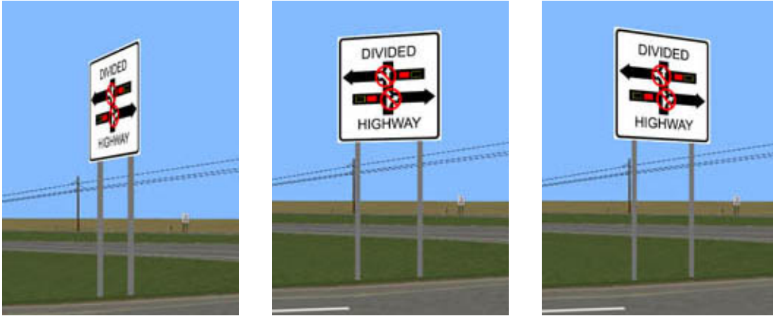
Figure 16. Example of an image set (Icon sign viewed from P_n ) shown to participants when they were asked to rank the angles in terms of how well they map information from the sign to the roadway conditions. The images depict a sign parallel (=), 45 degree, and perpendicular (+) angle conditions.
