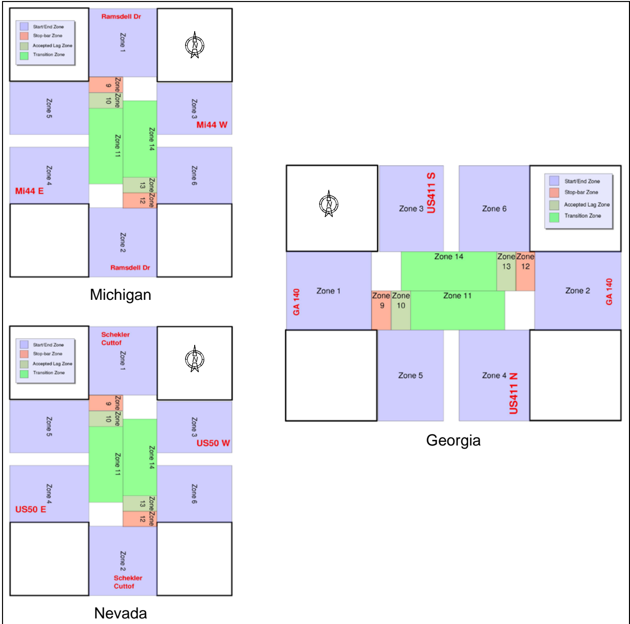
Figure 32. Position zones for rural, non-median separated highway intersections in Michigan, Georgia, and Nevada.
