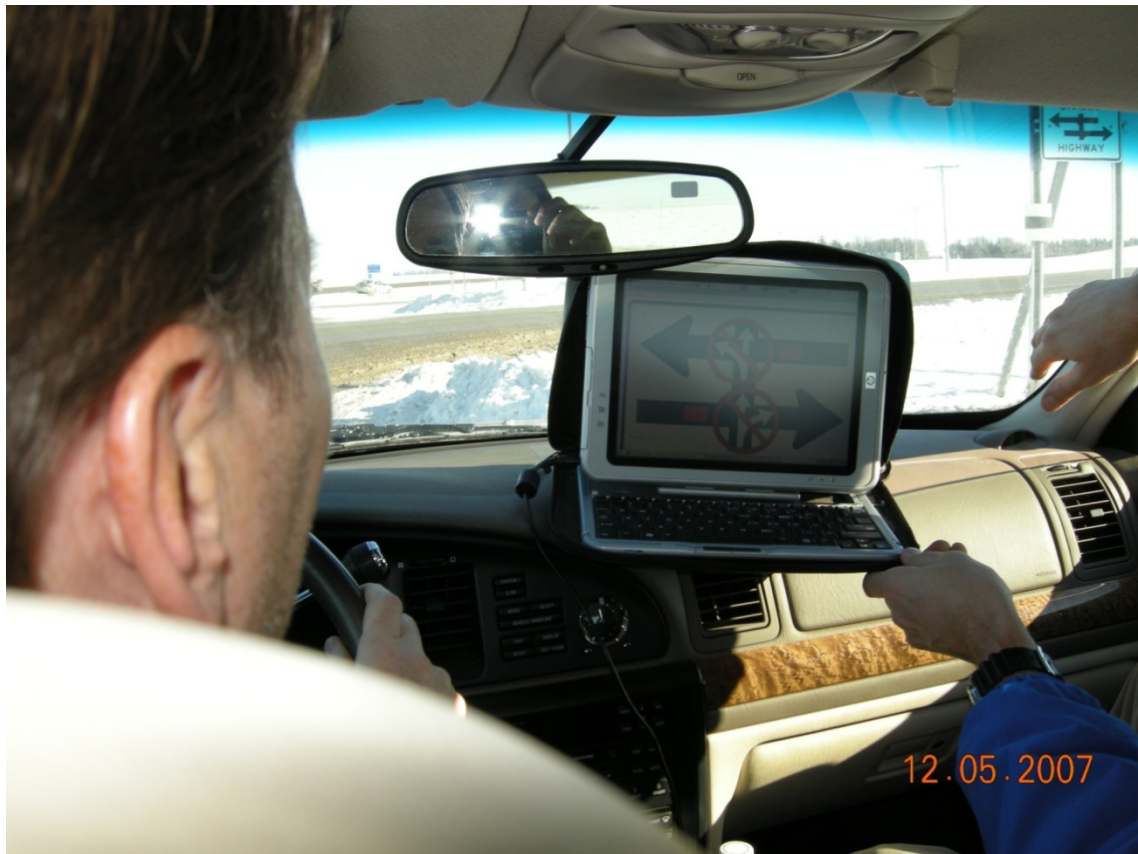
Figure 24. Alert and warning validation testing at Minnesota research intersection. Tablet PC is provided state map data, and is controlling the content of the driver interface, updating every 100 msec.
