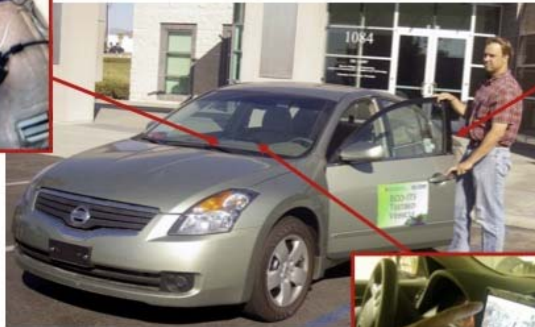
On-board computer interfaces with the vehicle CAN bus, navigation system, and wireless communications system
