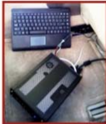
On-board computer interfaces with the vehicle CAN bus, navigation system, and wireless communications system
