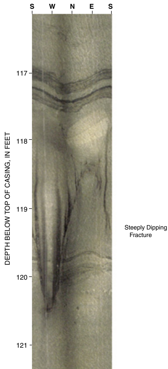
Figure 12. Optical-televiewer image of the flow zone near 119 feet in borehole RD-46A, Rocketdyne Sanat Susana Field laboratory, Ventura County, California.
