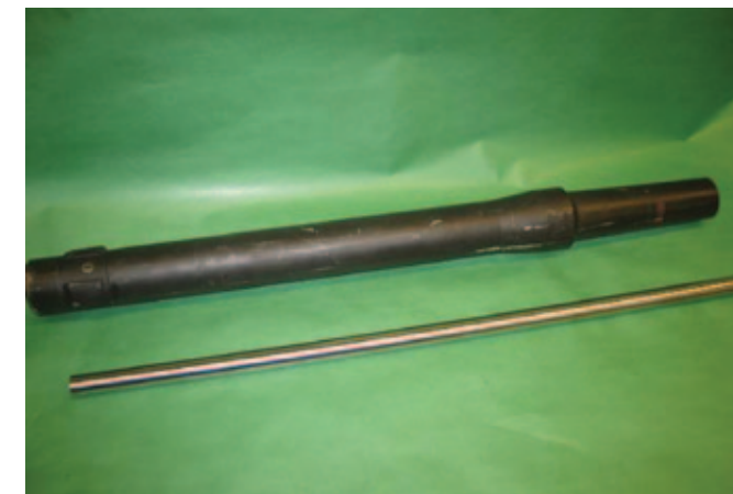
Liner and Barrel: The Stellite 25 liner was bonded to the truncated M242 gun barrel with the GLEEM process.
