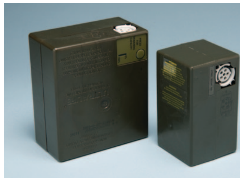
Advanced batteries with high specific energy being developed and evaluated for Soldier and communication applications.
