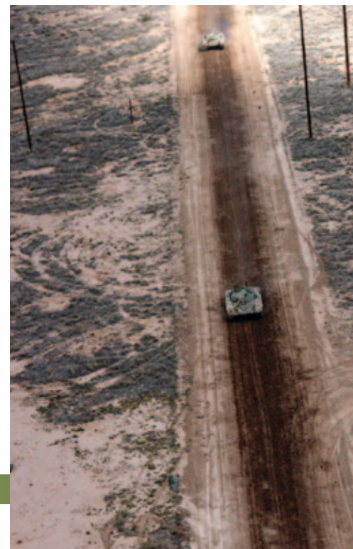
Two T-72s are driven on a test track to measure the IMS Scorpion response.
