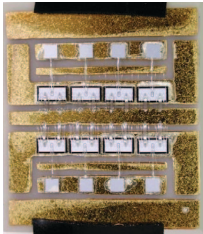
Bi-directional solid-state circuit breaker substrate populated with silicon carbide JFETs and silicon carbide gate resistors.
