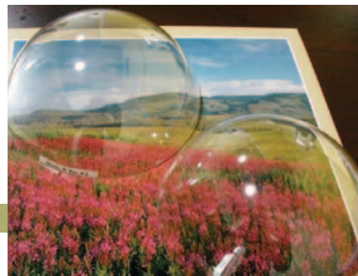
Sintered spinel domes for Joint Air to Ground Munitions (JAGM) Army/Navy, and small diameter bomb dome Air Force.
