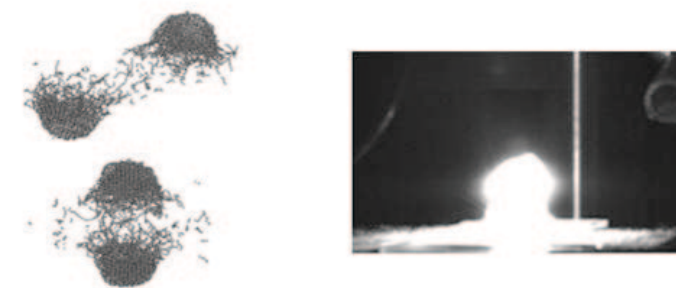
Figure 2. (left) Quantum mechanical simulations of two colliding nanodiamond particles, showing the significant spall and surface fragmentation. (right) Laser ignition of a conventional energetic material mixed with nanodiamonds.
