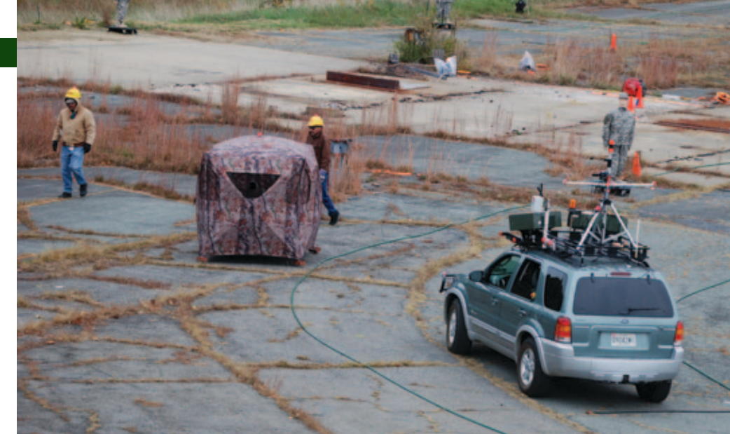
Detection, tracking, and avoidance of humans by an autonomous UGV during experiments conducted at the National Institute of Standards and Technology facility in Gaithersburg, Md.
