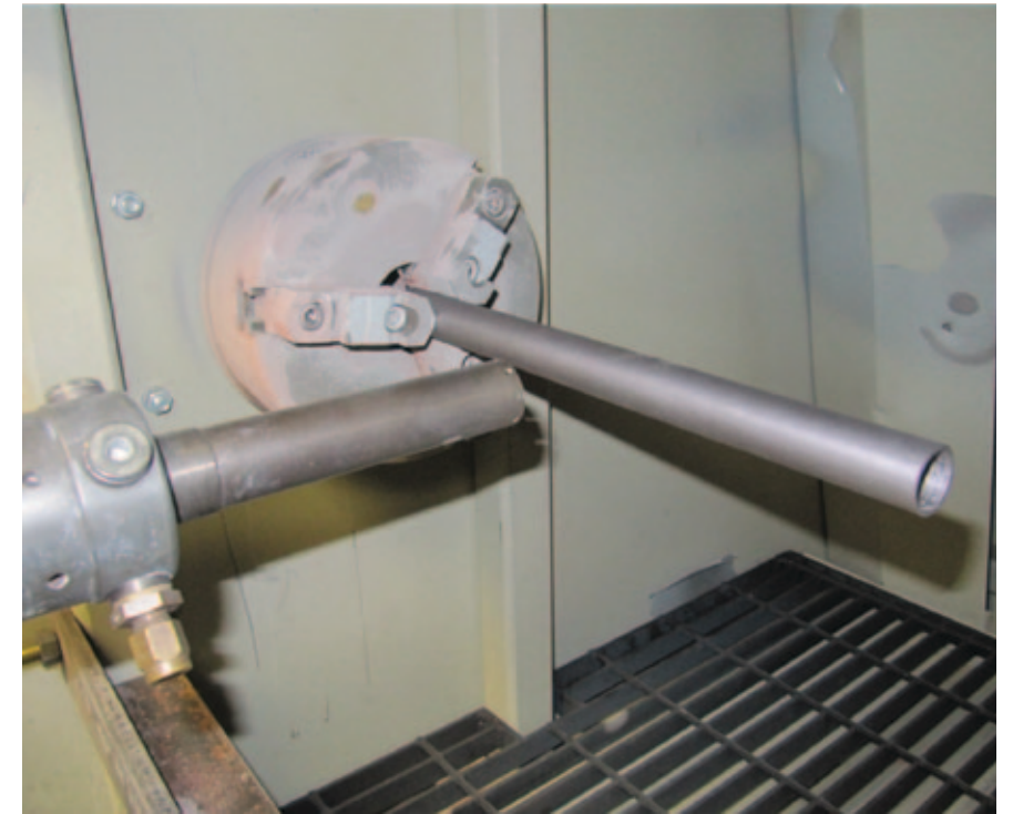
Cold spray consolidation of a tantalum tube.
