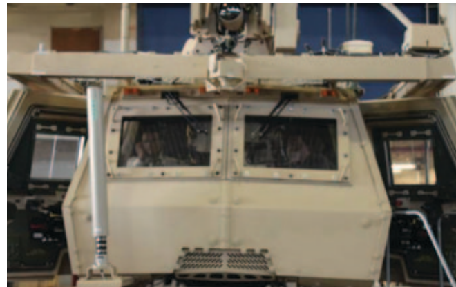
Spinel based transparent armor on FMTV 1083A1 P2 for TARDEC/ARL TWVS ATO demonstrator undergoing testing.
