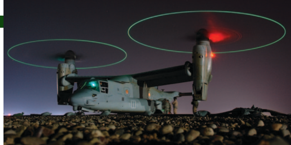
The V-22 Osprey is a multi-mission, military tiltrotor aircraft capable of vertical take-off and landing (VTOL).
