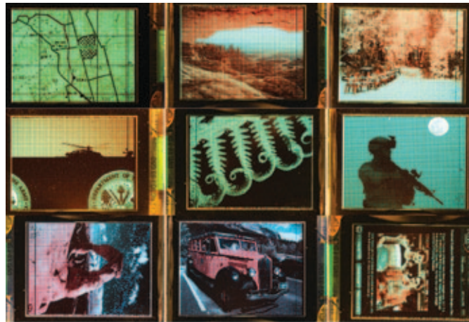
An array of flexible Color Emissive Displays developed at the Flexible Display Center. ARL contributed to the process development.
