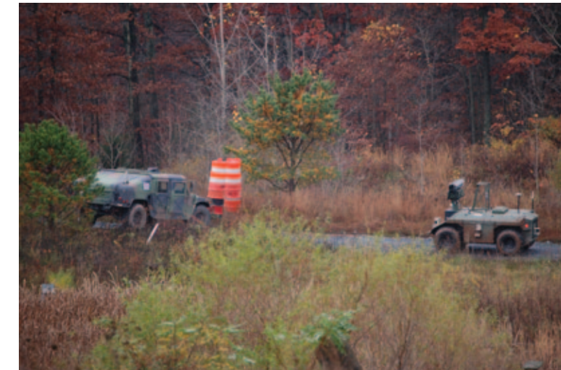
Unknown obstacles are sensed and data is incorporated for hierarchical planning as part of the Robotics CTA capstone experiment at Fort Indiantown Gap, Pa.
