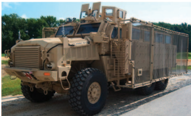
TOPS System installed on MRAP 6 X 6.
