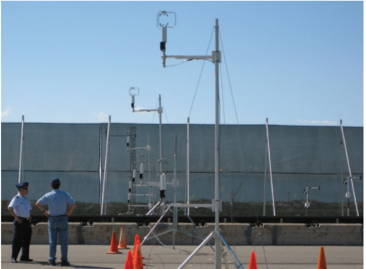
Dr. Wang of ARL examines sonic anemometer instrumentation for validation of the 3DWF model. The 3DWF was used to design the new wind barriers for the Air Force High Speed Test Track at Holloman Air Force Base (shown in foreground).
