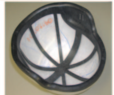
Graphite/epoxy stiffener applied to a polyethylene/aramid helmet.
