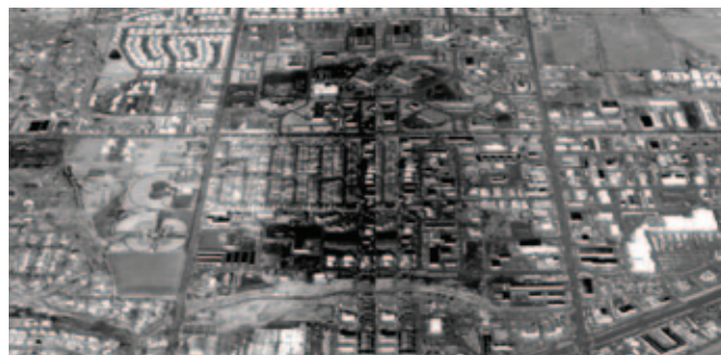
Aerial image taken by two one-megapixel C-QWIP FPAs operating simultaneously, which shows their ability in helicopter pilotage and large area surveillance.
