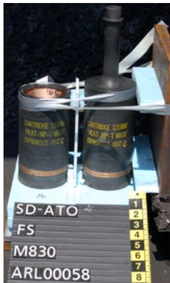
Experimental Set-up for Sympathetic Detonation Scenario on Munitions.
