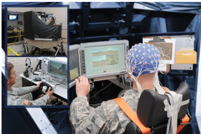
The Ride Motion Simulator (RMS) at TARDEC's Ground Vehicle Simulation Laboratory provided the ARL-led research team with unique capabilities to enhance the realism and increase the impact of research on neurotechnology development.
