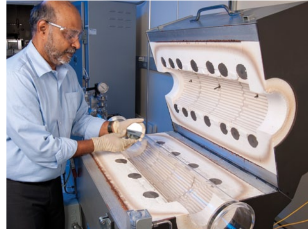
Dr. Priyalal Wijewarnasuriya inspects a TCA annealed 3-inch wafer from a large area annealing furnace.
