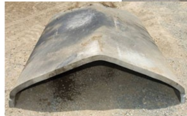
The MAK after the blast test event. The MAK had a permanent deformation of less than 1 inch.
