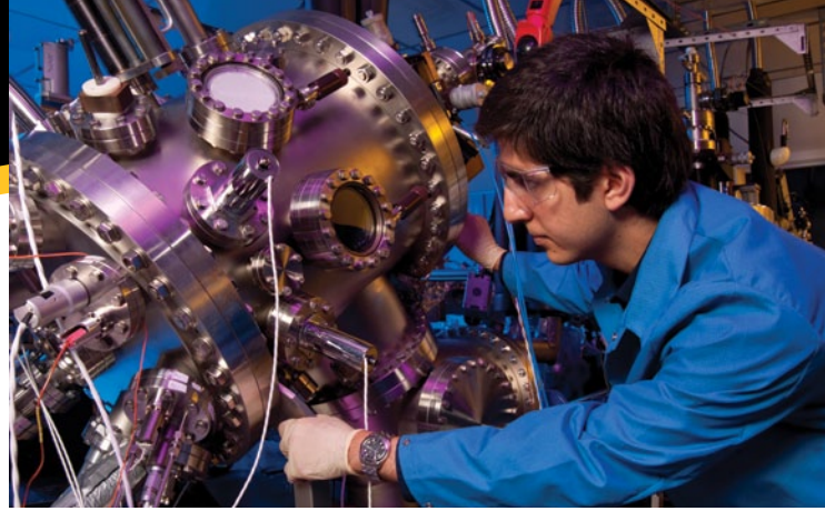
Sina Simingalam operates a molecular beam epitaxy (MBE) chamber for the growth of MCT on a large area Si substrate.
