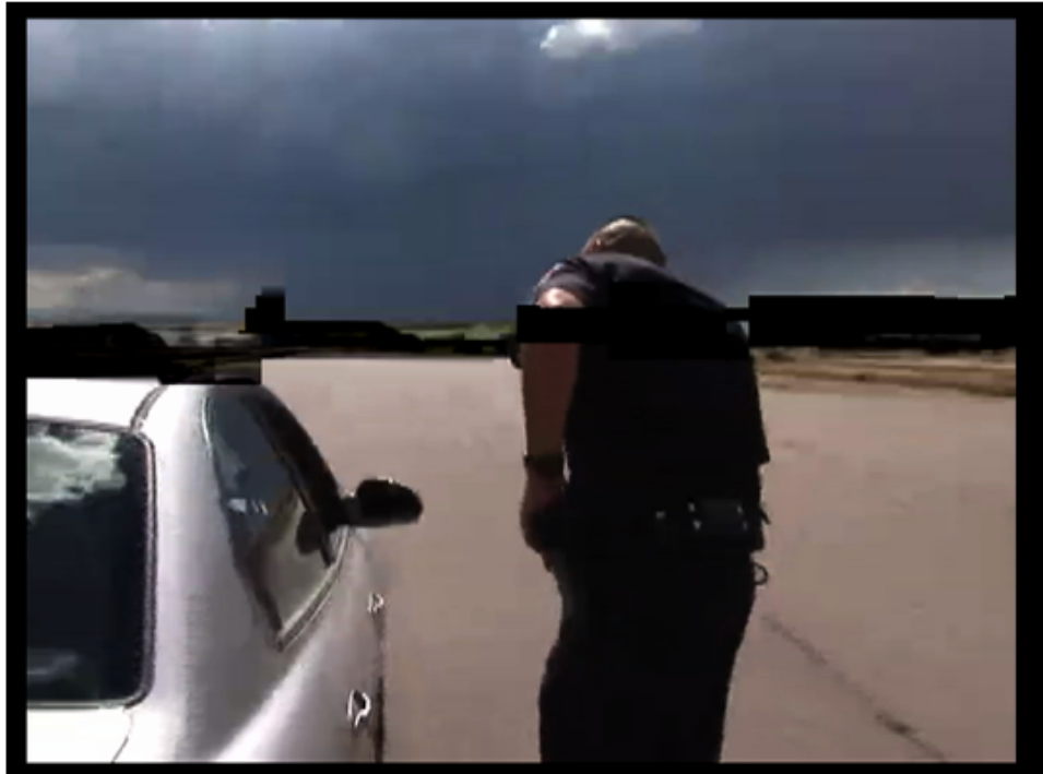
Figure 5: PS1 H.264 HRCs with 0.1 Percent Packet Loss (No EC) Example
