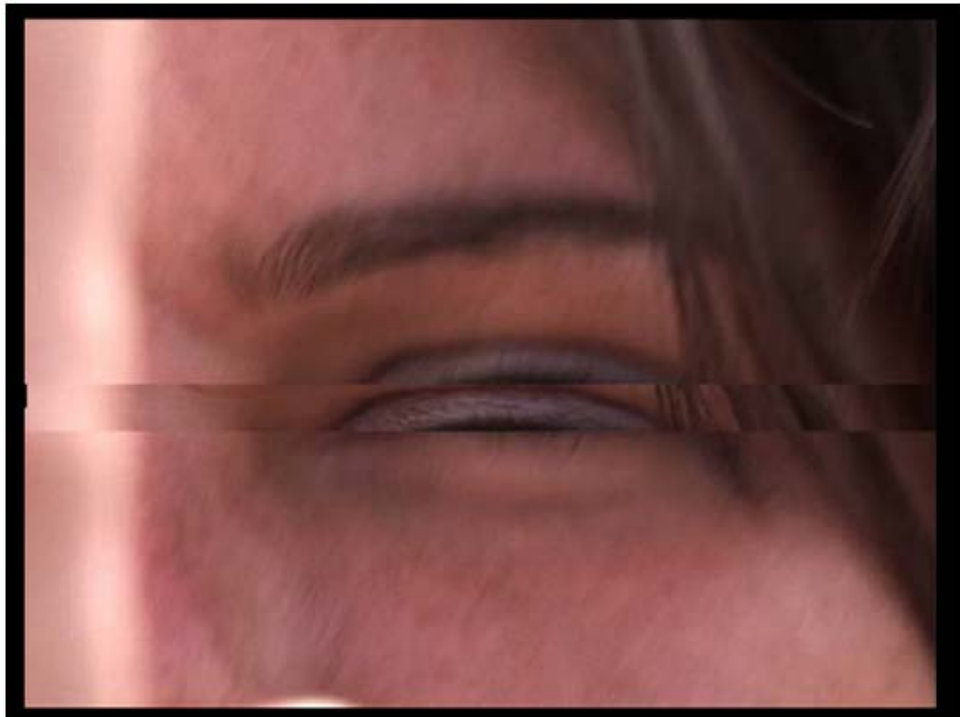
Figure 4: PS1 MPEG-2 HRCs with 0.1 Percent Packet Loss (No EC) Example
