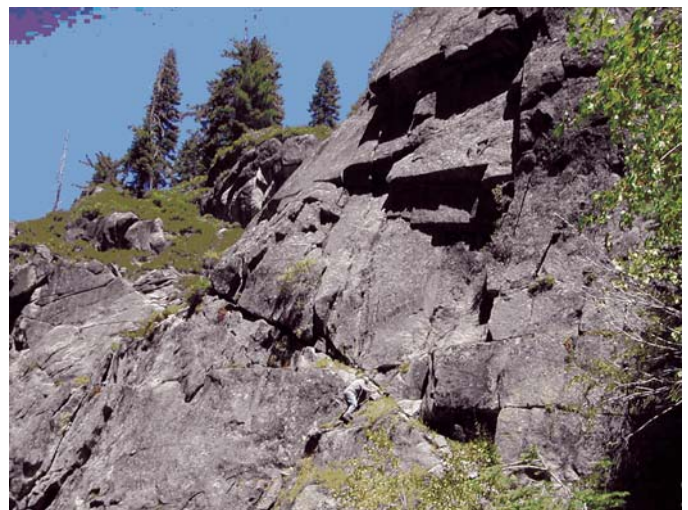
Figure 10. Examining geologic material, numerous joint sets, and local instability along eastern side of upper LeConte Gully west of Glacier Point above Yosemite Valley, Yosemite National Park, California.
