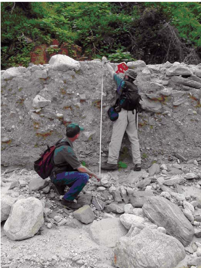
Figure 3. Measuring thickness of a recent debris-flow deposit along a stream channel in northern coastal Venezuela (Larsen and Wieczorek, 2006).
