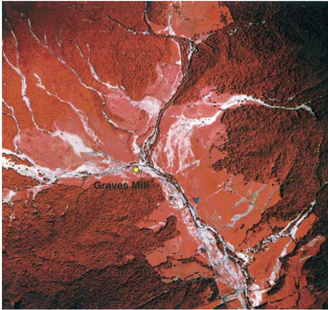
Figure 6. False-color infrared photography showing recent debris flows and flood effects in bright tones (white) with areas of unaffected forest (dark red) and grassland (pink) in Graves Mill, Madison County, Virginia (Wieczorek et al., 2000).
