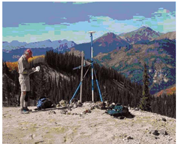
Figure 13. Slumgullion landslide station with radar corner reflector and GPS monitoring antenna, providing ground truth for InSAR measurements (Parise et al., 2004).
