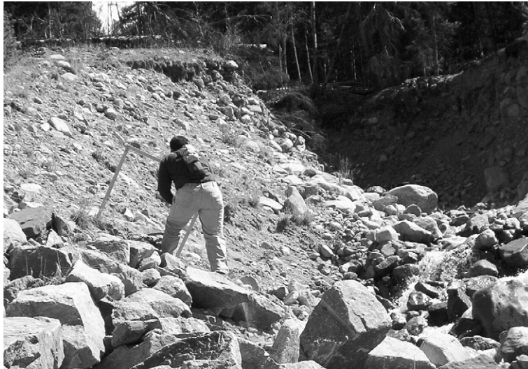
Fig. 2. Photograph showing the use of the slope profiler, advancing one length at a time across a scoured debris flow channel, recording the angle of inclination for each length.
