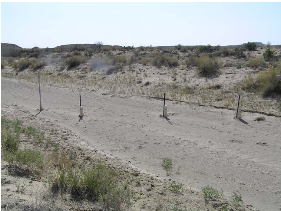
Photo 2 Surface water samplers located along Pinabete Arroyo, referred to as “Lower Pinabete”
