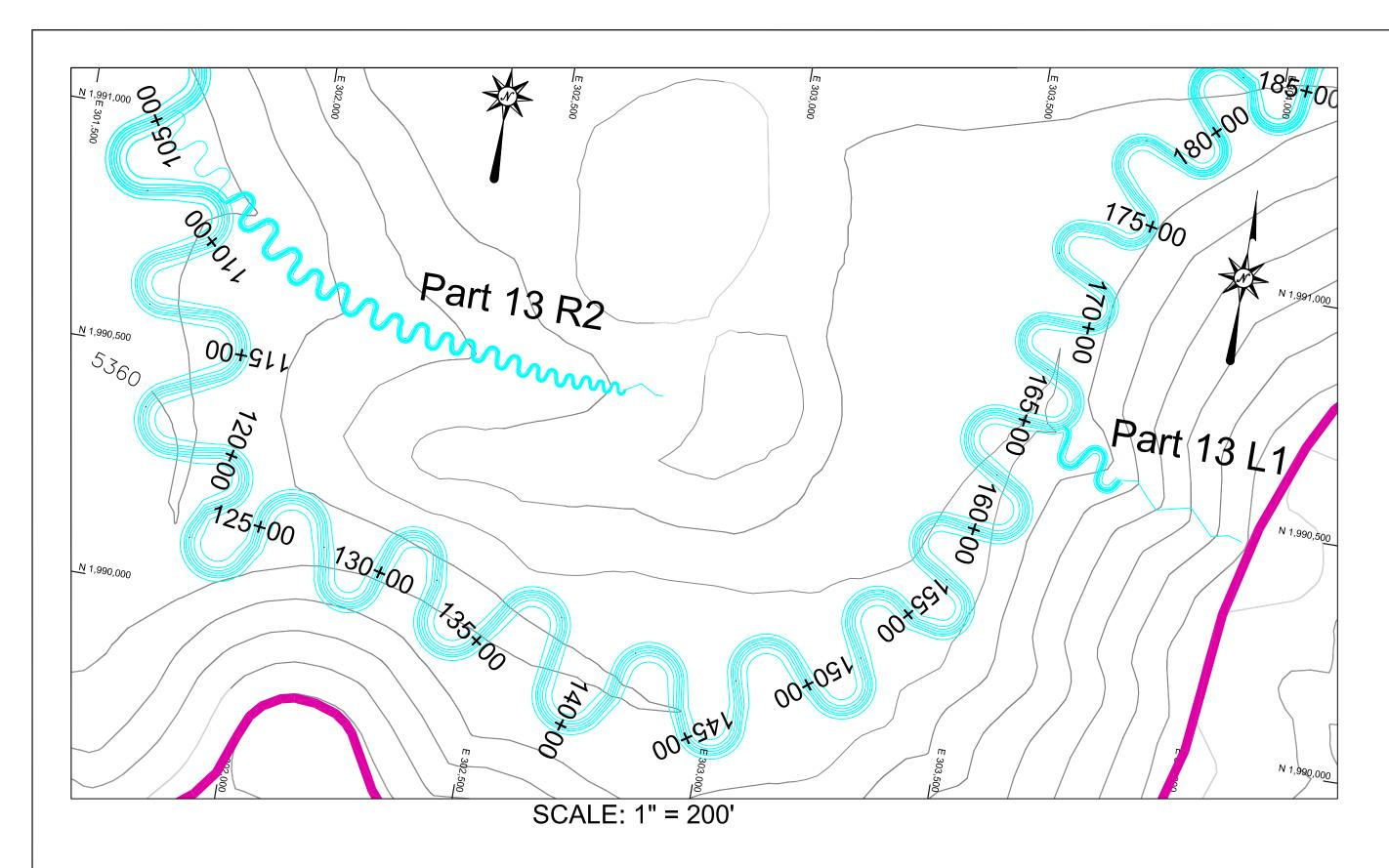
NOTE: PRIOR TO CONSTRUCTION, DESIGN CONTOURS WILL BE MODIFIED TO ACCOMODATE CHANNEL MEANDERS.
