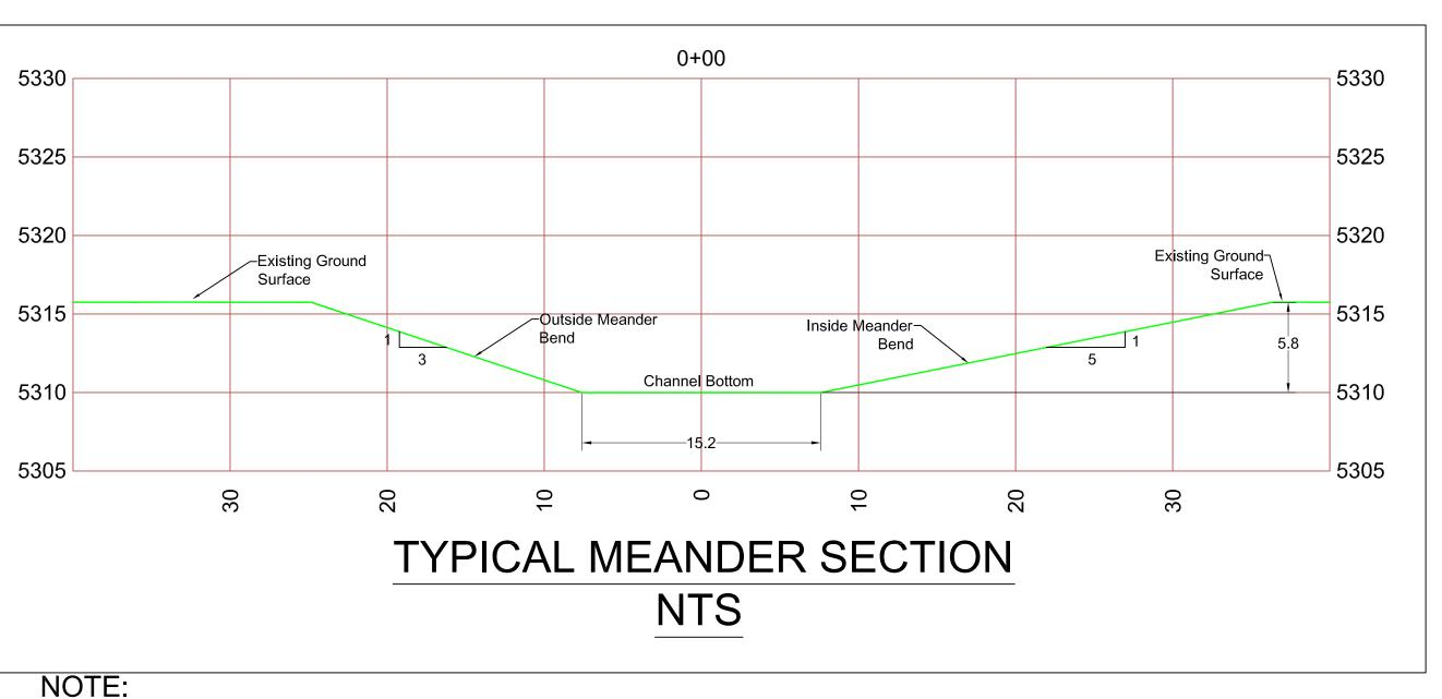
CHANNEL BOTTOM WIDTH RANGES FROM 15.2 FT AT STA 0+00 TO 13.6 FT AT STA 61+00. CHANNEL DEPTH RANGES FROM 5.75 FT AT STA 0+00 TO 5.16 FT AT STA 61+00.
