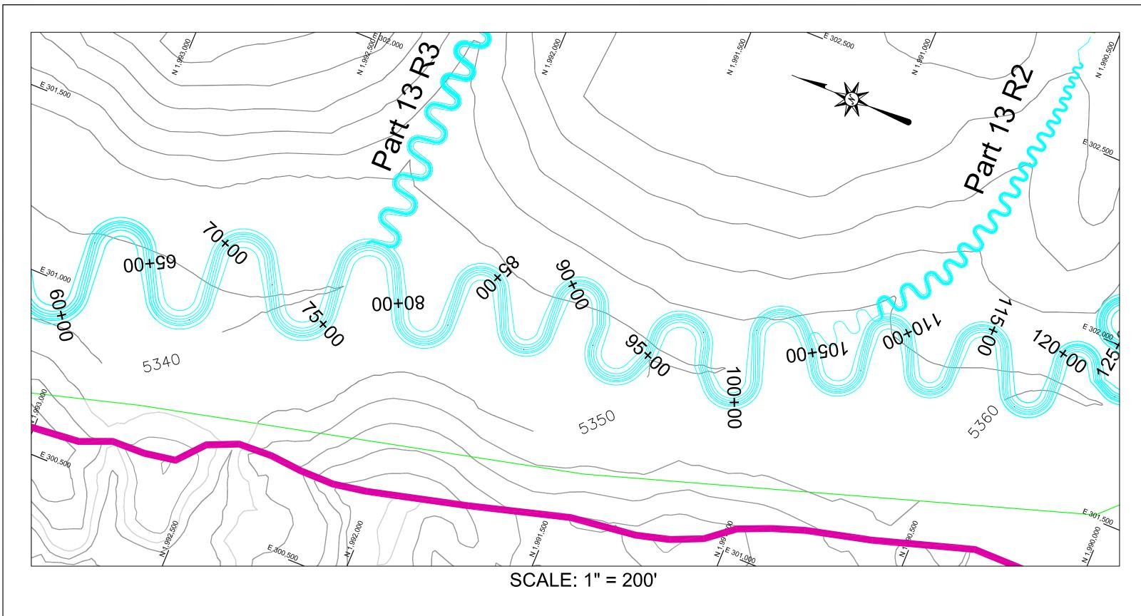
NOTE: PRIOR TO CONSTRUCTION, DESIGN CONTOURS WILL BE MODIFIED TO ACCOMODATE CHANNEL MEANDERS.
