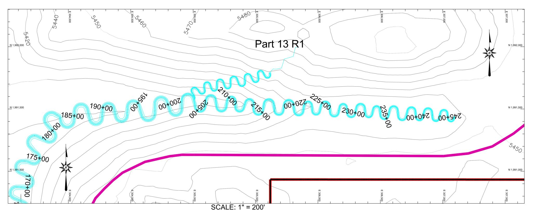
NOTE: PRIOR TO CONSTRUCTION, DESIGN CONTOURS WILL BE MODIFIED TO ACCOMODATE CHANNEL MEANDERS.
